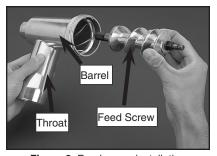
Figure 2. Feed screw installation
